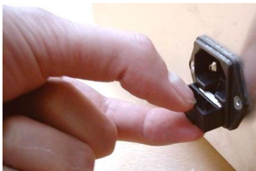
Figure 47: Renewal of the internal fuse
