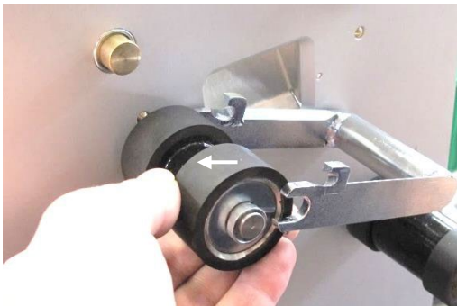
Figure 29: Pulling out the pressure roll
