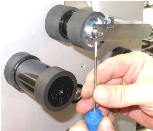
Figure 28: Unscrewing the pressure roll grub screw
