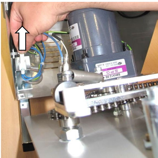
Figure 33: Disconnecting the motor plug
