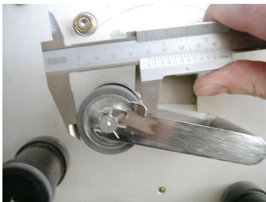
Figure 23: Checking the pressure roll diameter
