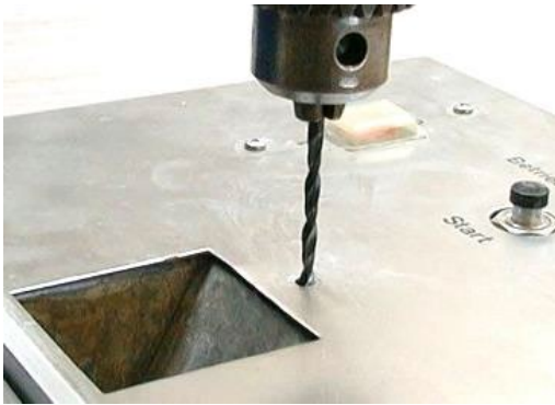
Figure 32: Drilling out rivets
