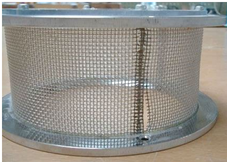
Figure 25: Damaged sieve drum
