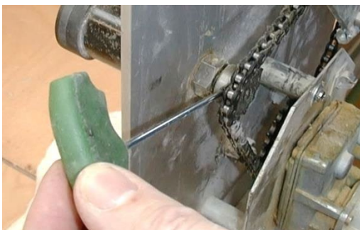
Figure 35: Unscrewing the chain sprocket
