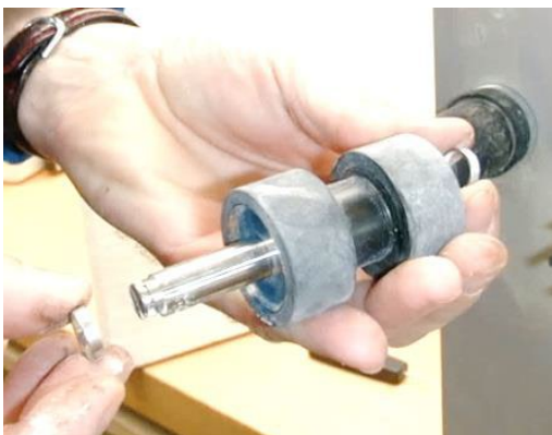
Figure 30: Place spacer rings onto the axle
