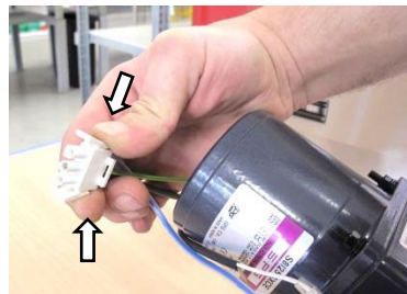
Figure 34: Pressing the motor plug together
