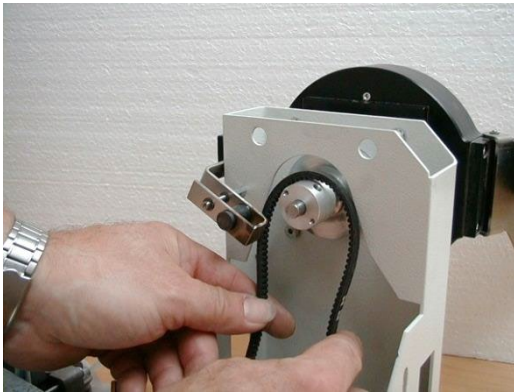
Figure 28: Remove/install the V-belt
