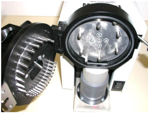
Figure 10: Clean milling chamber
