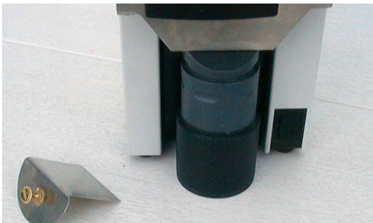
Figure 14: Place the sample dividing cup under outlet
