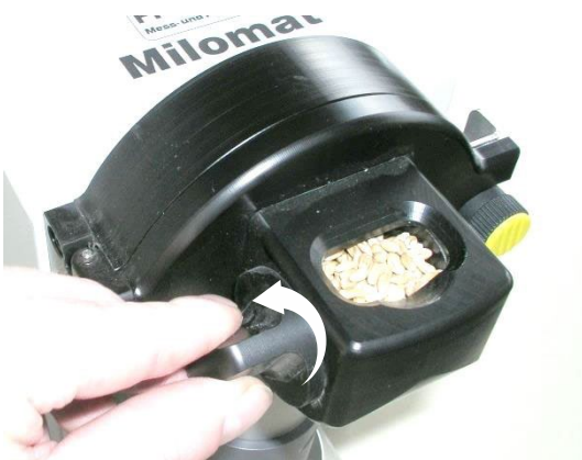
Figure 8: Empty filling hopper
