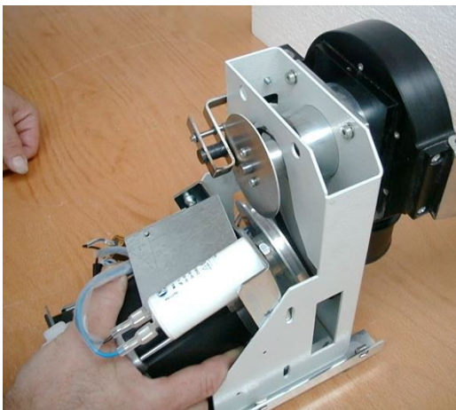
Figure 29: Insert the motor
